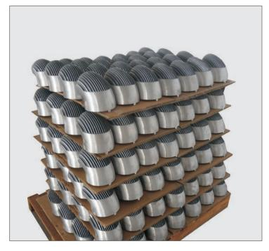
Aluminium die casting dies are run in cold chamber die casting machines. These machines are operated at the required temperatures and pressures to produce a quality part to net-shape or near net-shape specifications. Aluminium die castings can readily machined, anodized, painted or powder coated.
